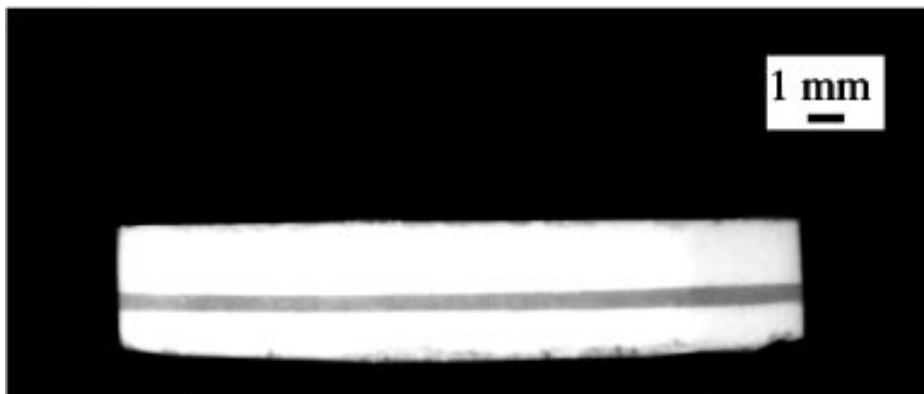
FIG. 1. Silver catalyst pellet. Dark band is Ag/ \alpha -Al 2 O 3 and white bands are \alpha -Al 2 O 3 .
